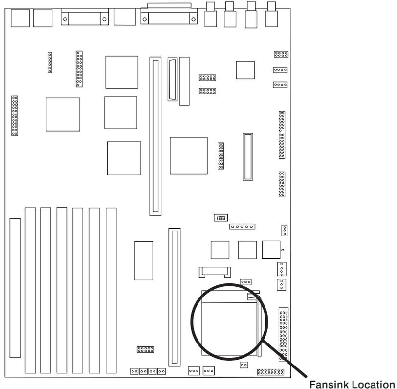
6. To remove a fansink with right-angle finger tabs, unclip the heatsink by pushing down and away on the fingertab. Remove the fansink assembly and discard.
